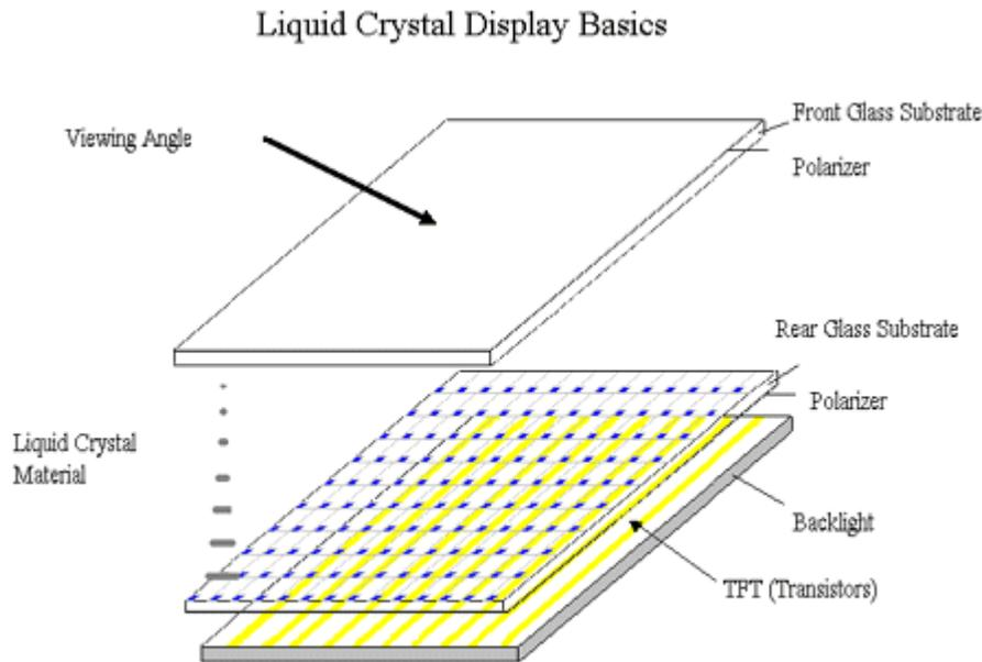
Note: The rear glass substrate contains both the LCD material and each pixel's transistor.
